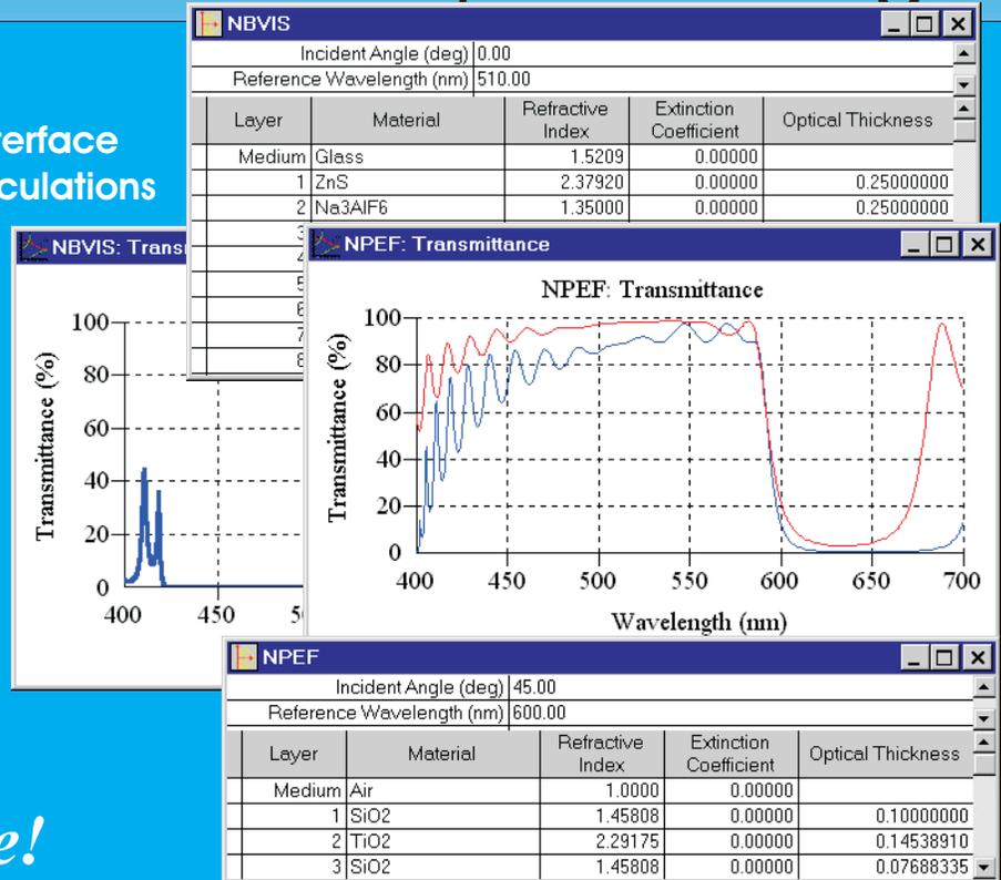
The Concise Macleod runs under any Microsoft Windows operating system and has a true Multiple Document Interface. It provides all that is essential for the performance calculation of an optical coating on a single surface, handling a wide range of performance parameters from ultrafast to color. It can refine designs using the Simplex method, investigate errors and produce admittance diagrams to improve understanding.
